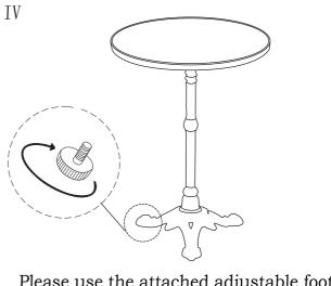
Please use the attached adjustable footglides to level the table on uneven surface.
