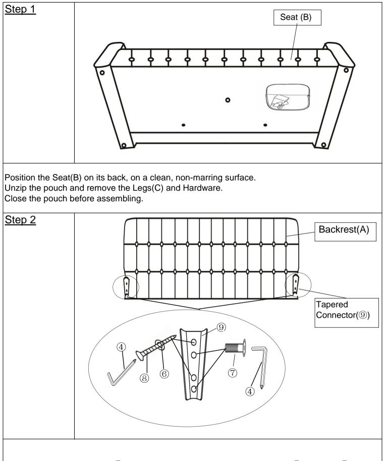
Attach Tapered Connectors(9) onto both sides of Backrest(A) using Bolts(7), Screws(8) and Washers(6) with Allen Key(4) as indicated in the diagram above.
