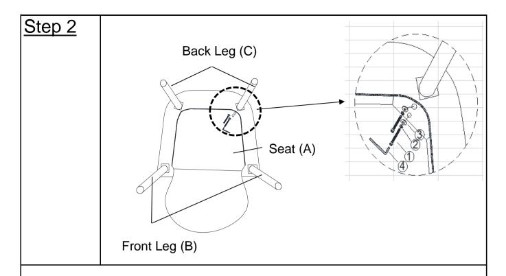
Align the mounting positions of the Back Leg(C) to Seat(A) and attach them using Bolts(1), Spring Washers(2) and Washers(3) with Allen Key(4) as shown above.
