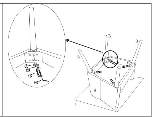
Insert the Leg(B) into the mounting position of Chair(A).
