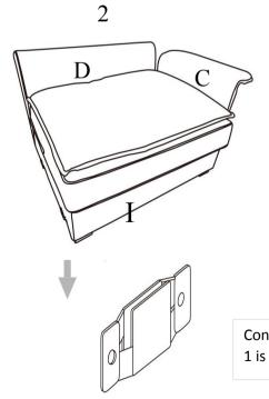
Connection mode: 1 is attached to 2
