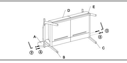
Attach Backrest(A) to Right Arm Panel(C) and Left Arm Panel(B) using JCBC Bolts(4) with Allen Key(3).
