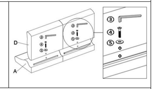
Place the Backrest(A) faceup onto a clean, non-marring surface. Attach Seater(D) to Backrest(A) using JCBC Bolts(4) and Washers(5) with Allen Key(3).
