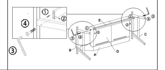
Insert Wood Dowels(①) into the Seater Rail(E) as pictured above. Attach Seater Rail(E) to Right Arm Panel(C) and Left Arm Panel(B) using JCBC Bolts(④) and Barrel Nuts(②) with Allen Key(③).
