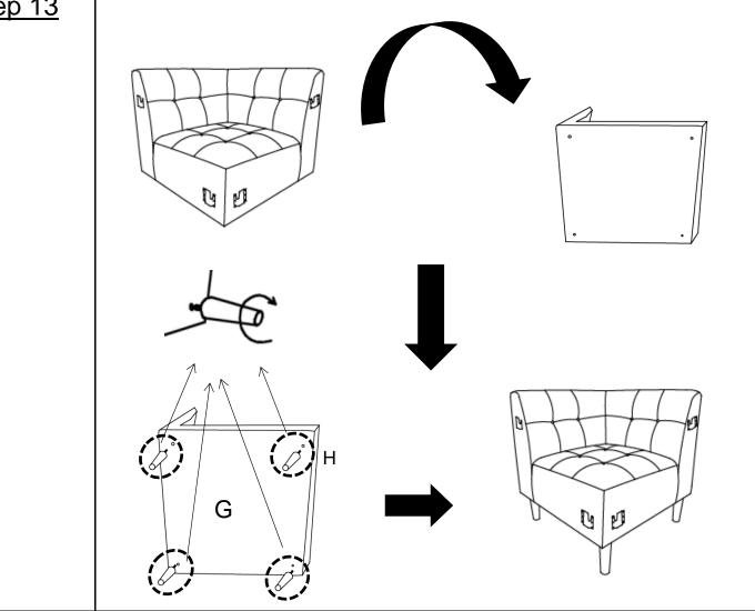
Install the Wood Legs(H) onto the bottom of the Corner Base by placing one  $Gasket(\oplus)$  on the threaded stem.
