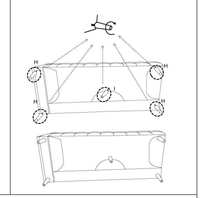
Install the Wood Legs(H) and the Middle Wooden Leg(I) onto the bottom of the Sofa by placing one Gasket(①) on the threaded stem.
