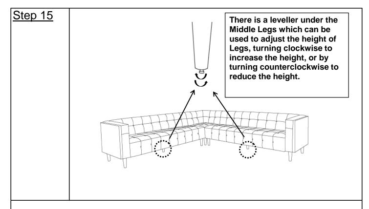
Note: If the sofa is unstable, you can adjust the levellers under the Middle Wooden Leg with Plastic Gasket(I) to make it stable.
