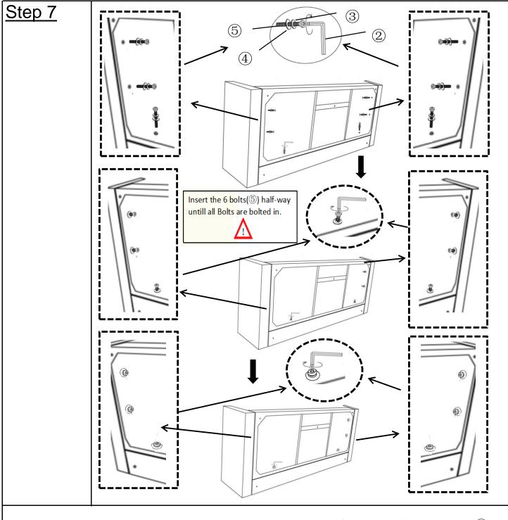
Using the Allen Key(2) secure Backrest(A) to the bottom of Seat Base(B) with Bolts(5), Spring Washers(3)and Washers(4).
