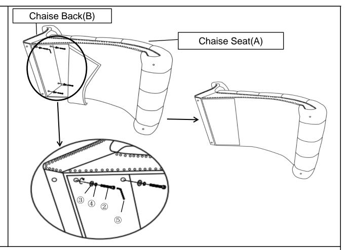
Install the Chaise Back(B) into the bottom of the Chaise Seat(A) using Bolt (②),Spring Washer(④),Flat Washer(③) with the Allen Wrench(⑤). Tighten all bolts at all joints completely.
