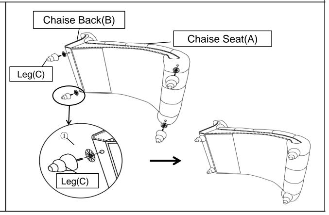
Install the Leg(C) onto the Chaise Seat(A) and the Chaise Back(B) by placing a Washer Ring(1) onto the stem. Insert the threaded stem into the threaded hole at each corner of the bottom of the Chaise Seat(A) and the Chaise Back(B). Tighten the Leg by turning clockwise, as shown.
