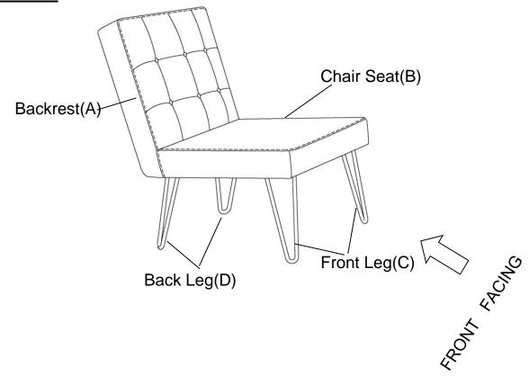
This Chair has multiple parts and may require up to 30 minutes to assemble. To give you an overview of the Chair, the above picture is to help you put the various parts into perspective. Please read through the instructions below to familiarise yourself with the parts and steps before assembly.
