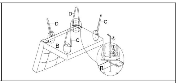
Attach Front Leg(C) to Chair Seat(B) using Bolts(1), Spring Washers(2), and Washers(3) with Allen Key(4) as shown in above picture.
