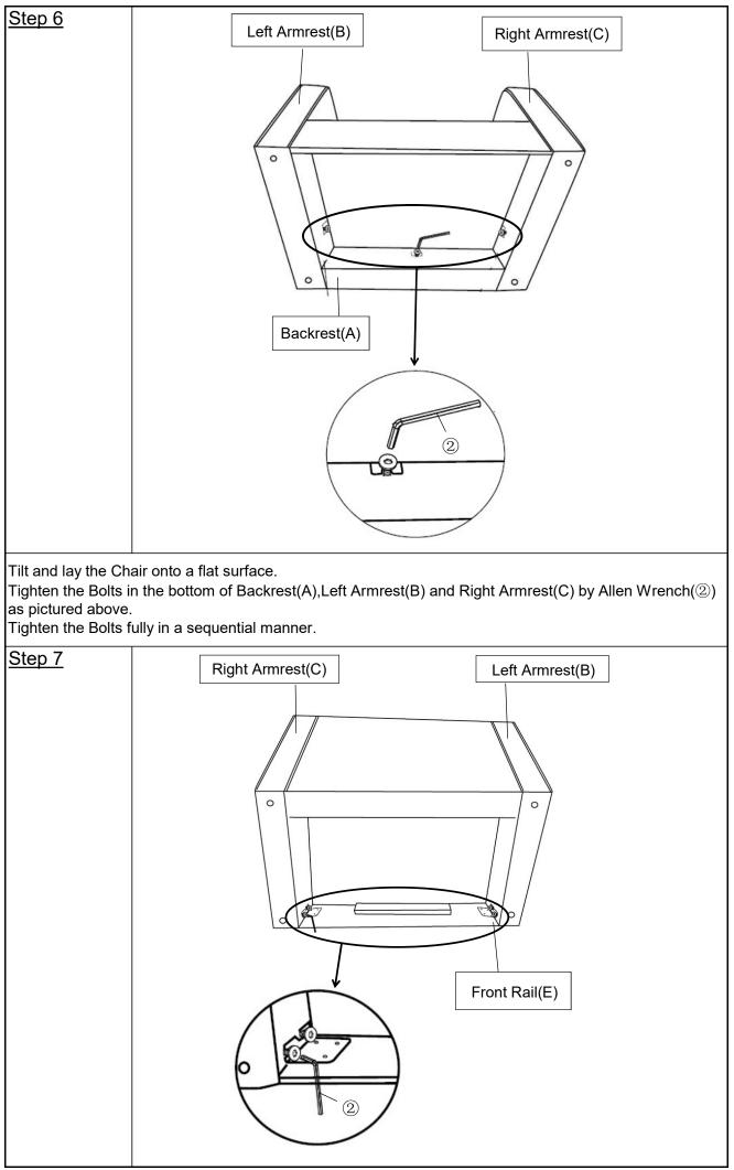
Change tilt and lay the Chair another side onto a flat surface. Tighten all the Bolts at the end of bottom Left Armrest(B) and Right Armrest(C) by Allen Wrench(②) as pictured above.
