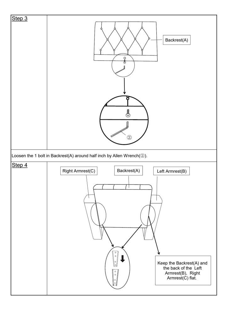
Slide the Tapered Connectors on the Backrest(A) into the Tapered Connectors on the Left Armrest(B) as shown in the picture.
