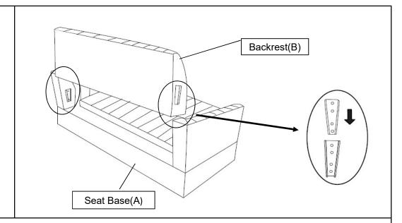
Attach the Backrest(B) to the Seat Base(A) by pushing the Backrest (A) downwards until the Backrest(A) is fully slotted and locked into position with Seat Base(A) as shown above.
