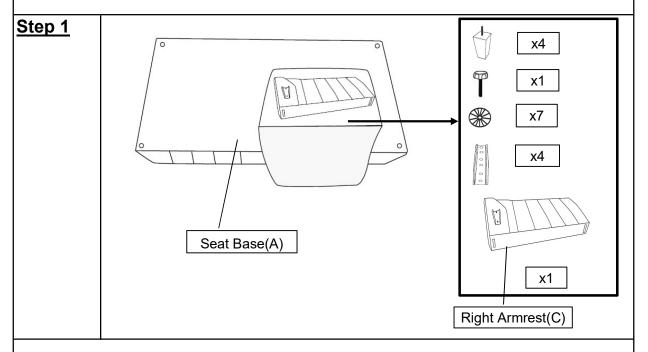
Position the Seat Base(A) on a clean, non-marring surface. Unzipper non-woven Fabric and Remove the Right Armrest(C), Leg(E) and Hardware package as shown above.
