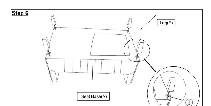
Install the Leg(E) onto the bottom of the Seat Base(A) by putting a Plastic Washer(①)(optional but improves security and tightness), onto the threaded stem. Insert the threaded stem into the threaded hole at each corner of the bottom of the Chair Seat(A). Tighten the leg by turning clockwise.
