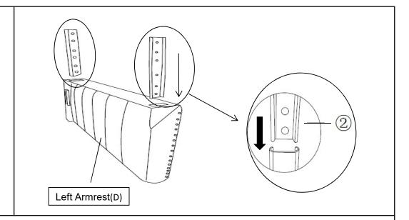
Position Left Armrest(D) on its back, put Double Head Insert(2) into Left Armrest(D) as shown above.
