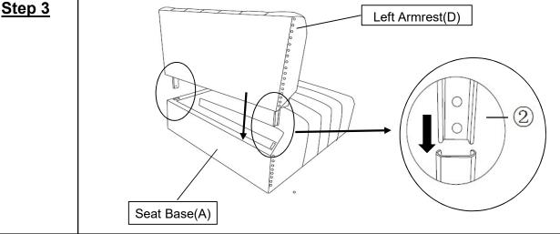
Slide the Double Head Insert(②) on the Left Armrest(D) into the Double Head Insert(②) on the Seat Base(A) as shown in the picture.
