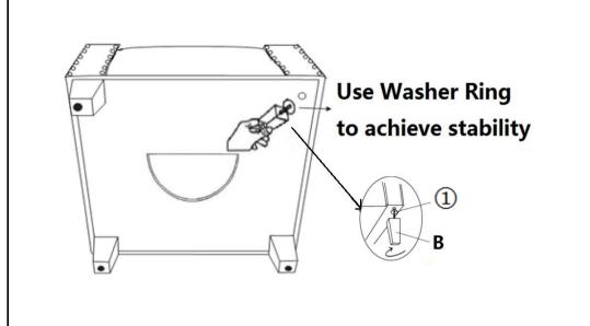
Install Leg into the Chair by putting a Washer Ring (1) on the threaded stem.
