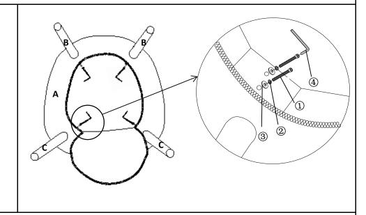
Insert the Back Leg(C) into the mounting position of Seat(A) and attach using Bolts(1), Spring Washers(2) and Washers(3) with Allen Key(4).
