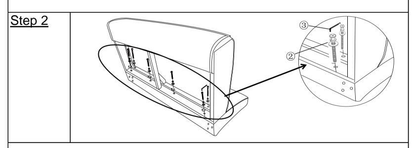
Put the Backrest onto a flat table or panel, insert the positioning dowels on the Seat panel to the mounting positionon the Backrest panel.
