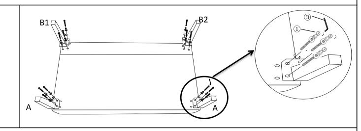
Install the legs(A&B1&B2) to Seat by using the Bolt Set (M6x30mm)(1) as shown. Use the Allen Key(3) to fasten all bolts. Caution:Do not fully tighten.
