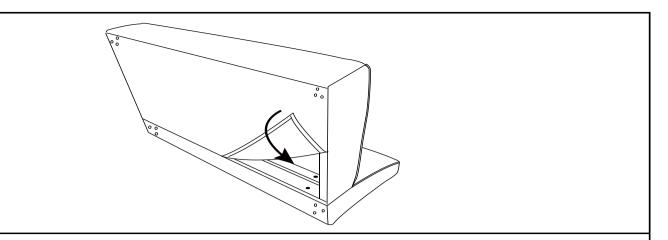
Place the velcro non-woven fabric cover back underneath the Seat(D)
