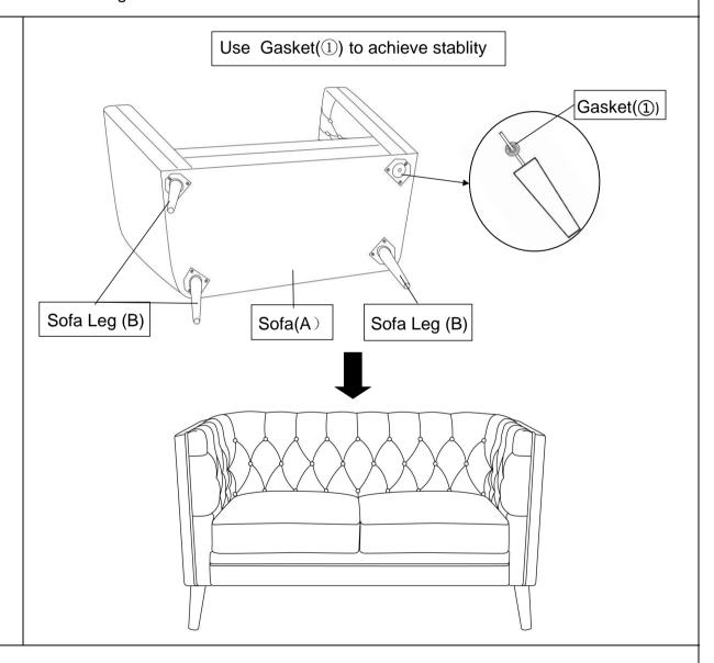
Install the Sofa Leg(B) at the bottom of the sofa by placing one Gasket(①) on the threaded stem.
