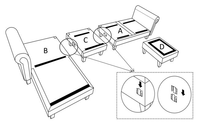
Connect the left seat base( $\bf A$ ) and the right seat base( $\bf B$ ) to the middle seat base( $\bf C$ ) as shown.
