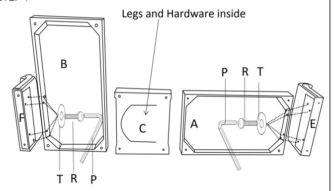
Attach the Right Arm (F) and the Left Arm (E) to the Seat Base using (8) M8x35mm screws (R) and (8) Ф22mm Washers (T), tighten with the M5 Allen Wrench (P).
