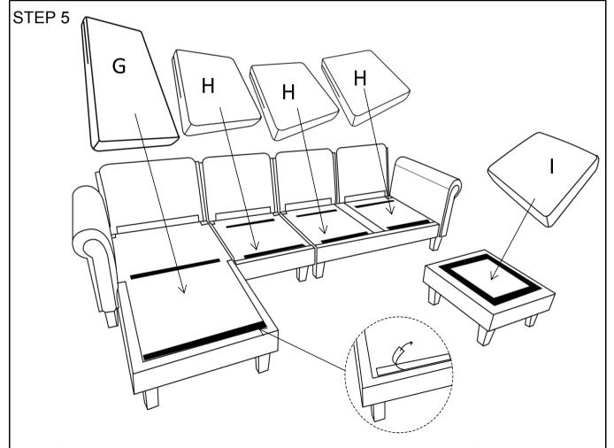
Tear off the Velcro protective cloth, then Attach the Seat Cushion into the Seat base as shown.
