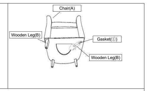
Install the Wooden Leg(B) into the bottom of the Chair(A) by placing the Gasket(①) onto the threaded stem.
