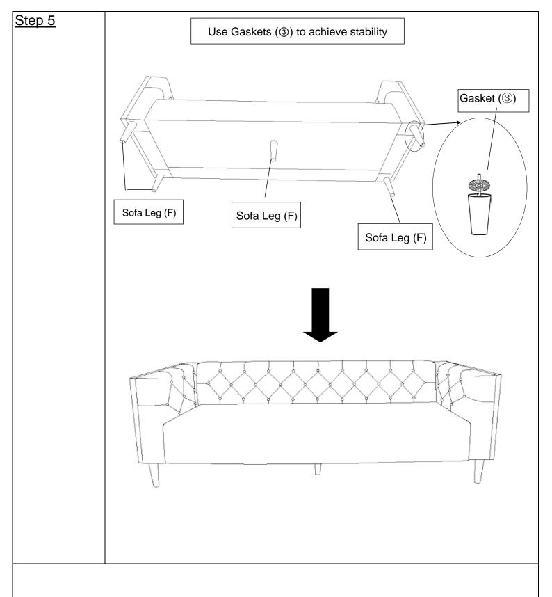
Install the Sofa Leg(F) to the bottom of the sofa by placing one Gasket(③) on the threaded stem. Then insert the threaded stem into the threaded mounting postion at one of the corners of the Sofa. Tighten by turning the Leg clockwise.
