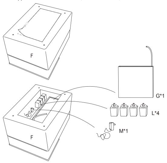
2.Zip up the zipper and screw the legs Part L to Part F,connect Power cable Part M to Part G.
