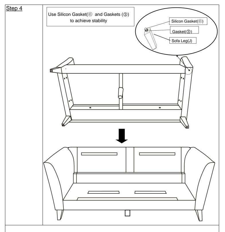
Install one of the Sofa Legs(J) into the Seat(E) by placing one Silicone Gasket (6) and one Gasket(3) onto the threaded stem.
