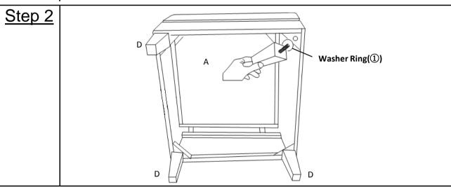
Install the Legs(D) into the bottom of the Chair Seat(A) by placing a Washer Rings(1) onto the threaded stem of the Legs.
