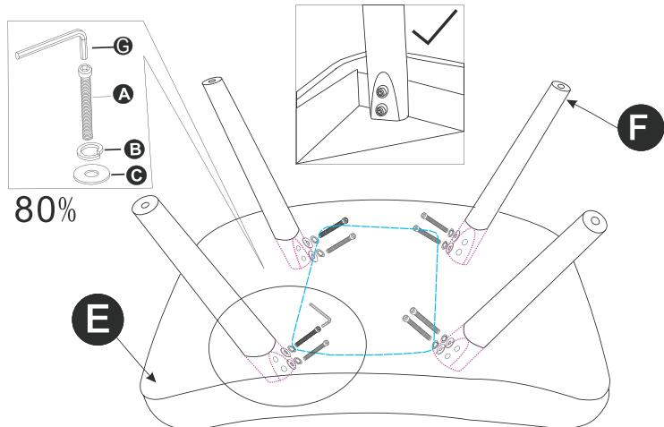
Please do **NOT** fully-tighten all screws before adjusting the balance of the whole footrest
