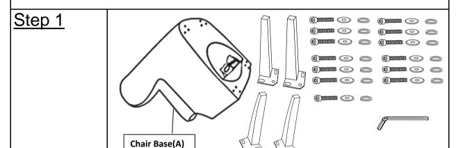
Position Chair Base(A) on its back as shown. (DO NOT place on surface that can scratch or damage upholstery.)
