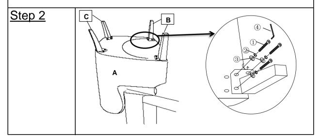
Insert the Front Leg(B) into the mounting position of Chair Base(A). Attach the Front Leg(B) using Bolts(1), Spring Washer Ring(2) and Washer Ring(3) with Allen Key(4), as shown.
