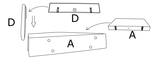
**DIAGRAM 4** (Assemble the Seat frame and Front baffle ) Connect the Seat frame(Parts A) to the Front baffle (Parts D) with the Washer (Hardware 1) and the Screws M6X35(Hardware 2) by Wrench(Hardware 7).
