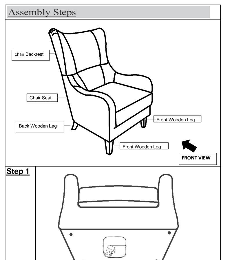
Position Chair Seat on its back, as shown, on a clean, non-marring surface. Unzip to open and remove the 4 Wooden Legs. Close pouch before assembling.
