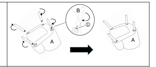
Install the Wooden Leg(B) at the bottom of the Chair by placing one Gasket(1) on the threaded stem.
