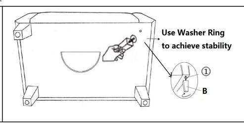
Install Leg into the Ottoman by putting a Washer Ring (1) on the threaded Stem and then Insert the threaded Stem into the threaded Hole at each Corner of the Bottom of the Ottoman(A).
