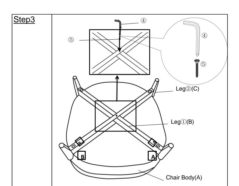
Attach the Leg<sup>②</sup> (Labeled "B") (C) to the bottom of the Leg<sup>①</sup> (Labeled "A") (B) using a Screw (⑤) and the Allen wrench(④) as pictured above.
