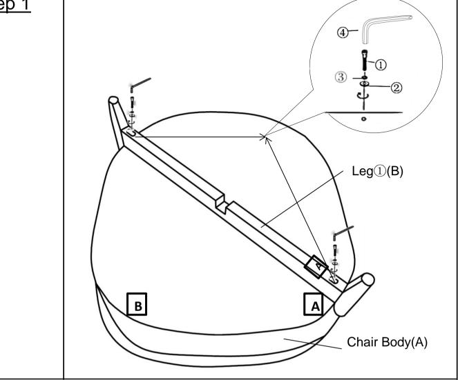
Place the Chair Body (A) on a clean and flat surface. Install the Leg① (Labeled "A") (B) using Bolts(①), Washers(②), Spring Washers(③) and the Allen Wrench (④) on the bottom of the Chair Body (A) as pictured above.
