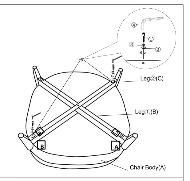
Install the Leg@ (Labeled "B") (C) using Bolts(@), Washers(@), Spring Washers(@) and the Allen Wrench (@) on the bottom of the Chair Body (A) as pictured above.
