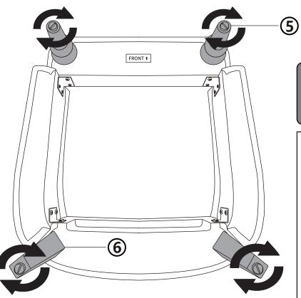
Note: Before installing the wooden foot, Remove the protective caseinstall firsit, Then cover with non-slip plastic sheet
