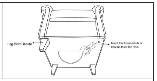
Install Wooden Leg(B) into the Chair(A) by putting a Washer Ring(①) on the threaded stem and then insert the threaded stem into the threaded hole at each corner of the bottom of the chair.
